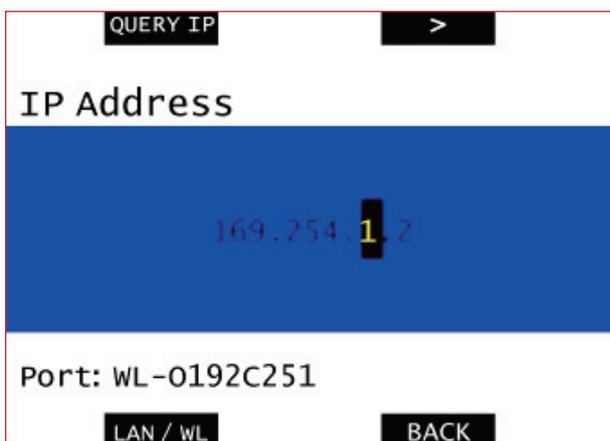
Press QUERY IP to get the IP address from the camera.
